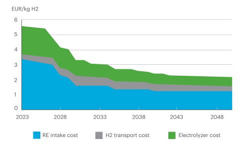
**Figure 3** Levelised cost of hydrogen split into renewable electricity intake, transport and electrolyser cost [Source: ILF]
