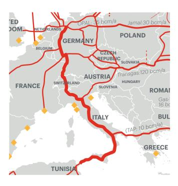
**Figure 6** Potential pipeline route for hydrogen transport from North Africa to North-West Europe [Source: ILF]
