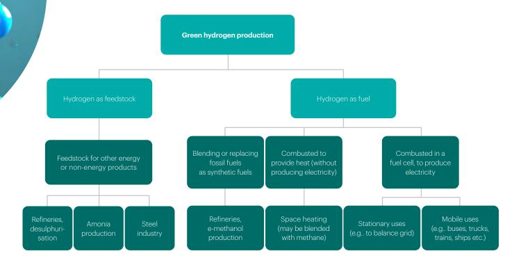
Figure 1 Classification of end-users of low carbon hydrogen
